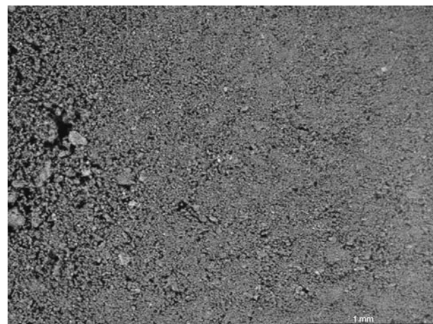
Figure 6 Matte – original sample after bacterial leaching and calcinations (using a Zeiss NU-2 microscope)
