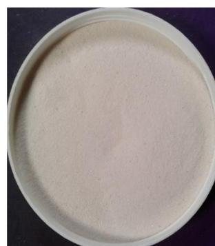
**Figure 2:** Sieved dolomite sample
