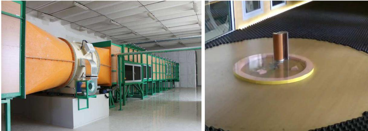
Fig. 2: The wind tunnel - BLWT STU and the experimental "S" model [6].
