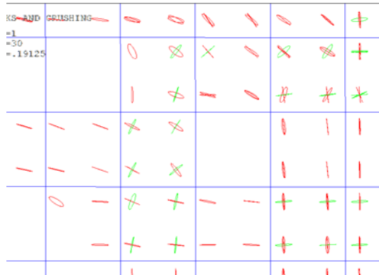
Fig. 9 Detail of crack pattern of homogenized macromodel
