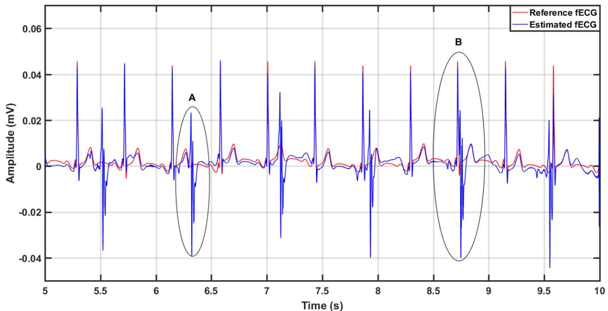
Fig. 7: The output of an adaptive filter using the RLS Algorithm.
