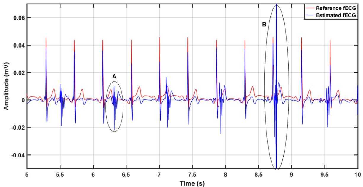
Fig. 6: The output of an adaptive filter using the LMS Algorithm.
