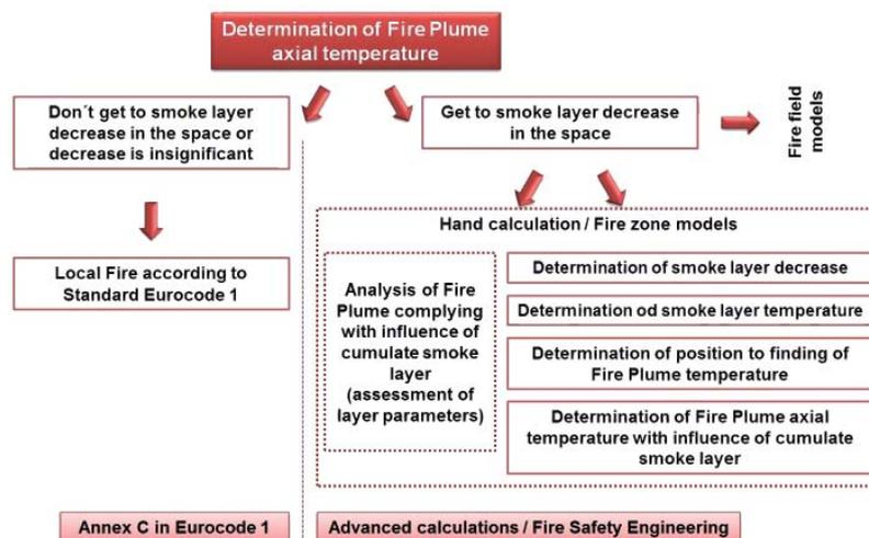
Fig. 3 The procedure for determining the axial temperature of the Fire Plume (Kučera and Pokorný, 2010)
