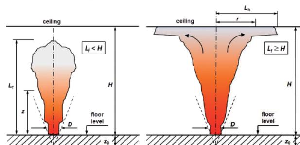
Fig. 1 Flames of fire in a confined space (Kučera and Pokorný, 2010)
