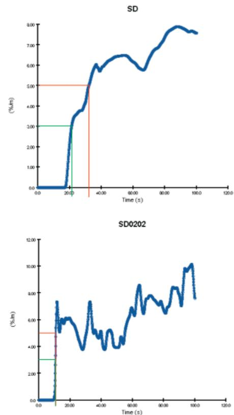
Fig. 5 Response time of detectors SD and SD0202 for 500 kW burner and  $W = 1 \times D$
