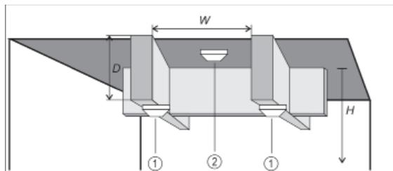
Fig. 3 Honeycomb structure considered by British standard (BS 5839-1:2013)
